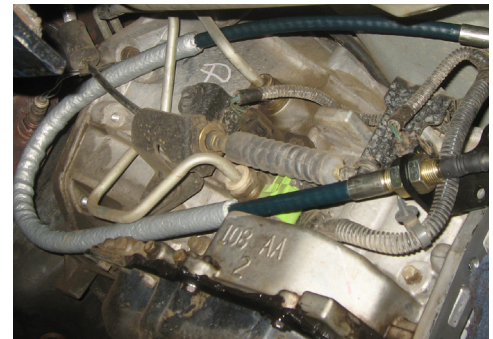
Figure 14: RubiCrawler Cable Routing
