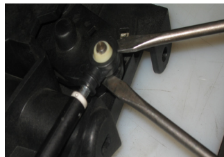
Figure 12: Rod End Removal
