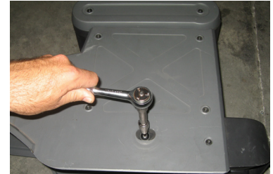
Figure 7: Rear Bolt Location
