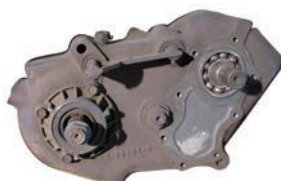
NP205 T/C figure-8 bolt pattern
