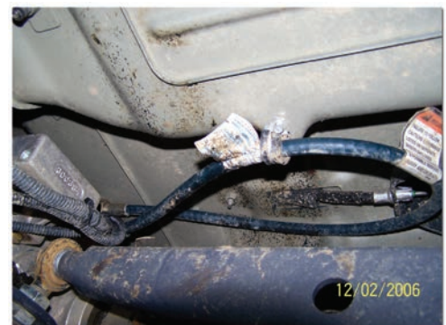
Jeep TJ 4 speed shifter located between the E-brake and the console (left) and the 4 speed cable routed on a Jeep TJ (right)
