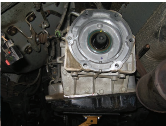
The 42RLE transmission rear housing after the stock transfer case has been removed.
