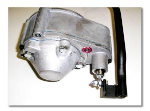
Both above photos illustrate the shift rod installation on the Saturn Overdrive. The shift rod must remain in close proximity to the overdrive unit for proper floorboard clearance. The configuration of some of the shifter rods are to avoid transfer case shifter lever interference.
