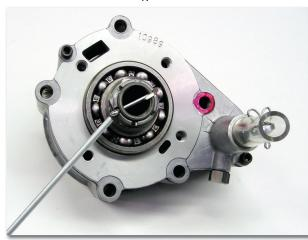
**Step C2**Remove the cotter pin that locks the nut to the spline shaft.
