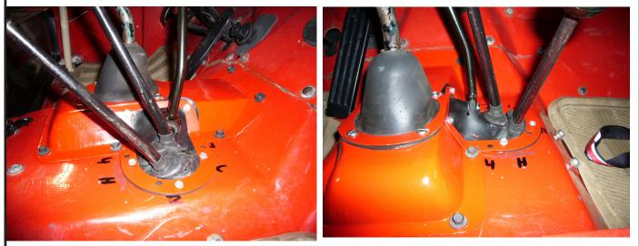
Saturn installed with a Dana 18 twin stick shifter
