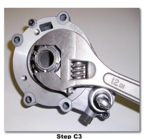
Remove the nut using a 12" adjustable wrench. The shift fork must be at the rear of the case, locking the unit in the overdrive position before the nut can be removed. Castle nut is torqued
