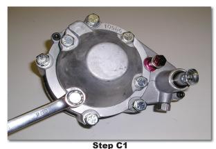
Using a 9/16" wrench, remove the 4 cap screws holding the bearing cap.
