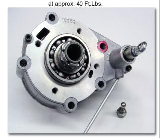
**Step C4**Remove the shift detent screw, ball and spring.
