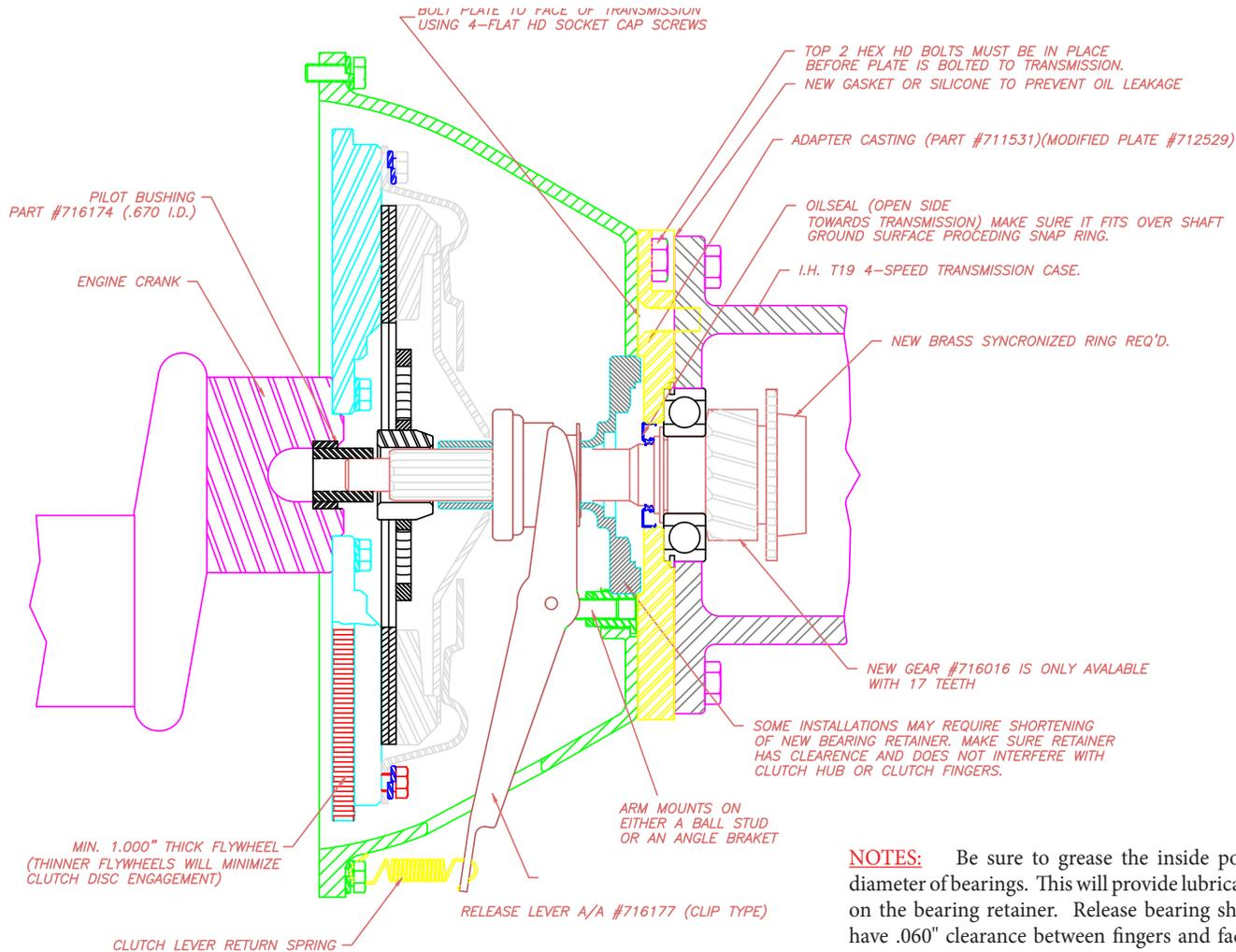
**NOTES:** Be sure to grease the inside pocket diameter of bearings. This will provide lubrication on the bearing retainer. Release bearing should have .060" clearance between fingers and face of bearing. Clutch disc should have .030" clearance between flywheel and disc when fully disengaged.
