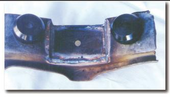
In order to mount the new adapter housing into the original Bronco crossmember, you will need to modify the crossmember for additional clearance. The new adapter housing is wider and will require a slight elongation on the bushing index holes of the crossmember.
