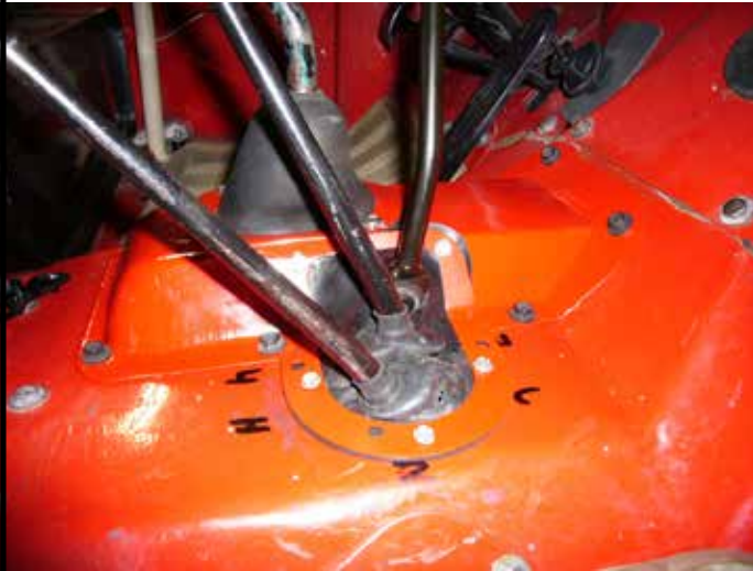
Saturn installed with a Dana 18 twin stick shifter
