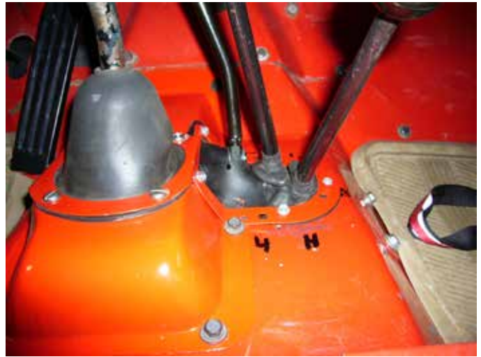
Saturn installed with a Dana 18 twin stick shifter
