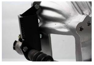
The new push rod has a ball end fitting that can be used up to the GM fork. To use the wedge connection, remove the ball fitting, thread on the new nut and install the wedge.
