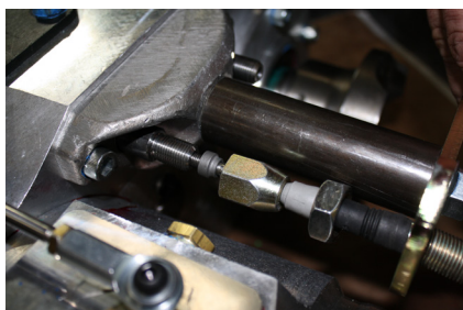
Once the cable nut has been adjusted, slide the nut cap over the shift rail and tighten to retain the cable to the shift rail. Shift the transfer case into low range (shift rail pushed inward) to set the outer cable housing.
