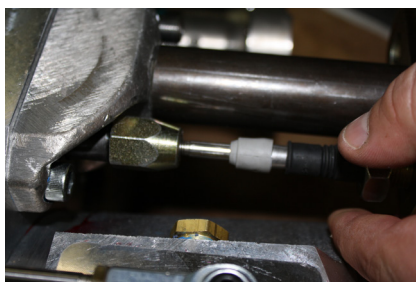
Once the cable nut has been adjusted, slide the nut cap over the shift rail and tighten to retain the cable to the shift rail. Shift the transfer case into low range (shift rail pushed inward) to set the outer cable housing.
