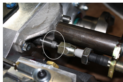
The cable should bottom out in the shift rail and the cable nut should be flush against the face of the shift rail.
