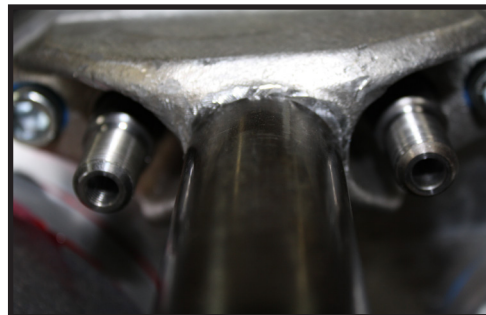
New shift rails with clearance holes drilled
