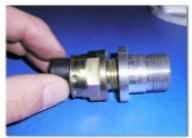
Remove the bushing after test fitting and then install the new reluctor sensor.
