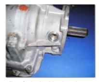
Test fit the bushing into the transmission housing. Make sure the bushing fits snug to the outside of the transmission. Note: You will have a small gap on the top and bottom side of this bushing, between it and the transmission.
