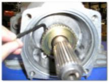
Tighten the 3 set screws of reluctor ring to lock it to the main output shaft. The allen wrench may need to be shorten to fit the set screws around the transmission case.
