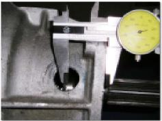
. After sensor hole has been drilled
