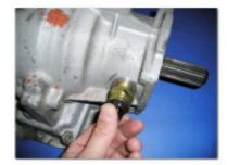
8. You will now need to install the bushing back into the transmission housing. The bushing will require RTV Blue silicone applied to seal the bushing to the transmission. Use just enough to form a bead around the outside of the bushing.
