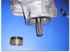
The clamp on reluctor gets installed onto the 4L60E output shaft and locked into position. If a 700R shaft is to be used, a different set collar in needed.
