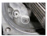
this transmission web. Once this hole location is located, drill a pilot hole with the 1/4" drill and work your way up until the 7/8" hole is obtained.
