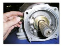
9. With the sensor and bushing set into the transmission, slip the wedge over the bushing so that the radius portion fits the inside contour of the case. Next, put Loctite thread retainer on the nut and then install the nut onto the bushing. The bushing will need to be slightly pulled out of the transmission to fit on the nut. Be careful not to move the bushing to much because you want to keep a good seal with the silicone.
