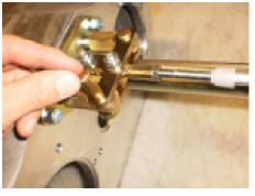
Loosely assemble supplied heim onto the 5/16"-24 cable threads. NOTE: The cable only mounts to the transfer case in one direction. Inspect the cable and find the end with a grove on in. The opposite end has a threaded section for mounting to the handle. Connect the groved end to the Heim joint. Attach the cable onto cable mounting bracket with supply U-bolt and 5/16"-24 thin locknuts.
