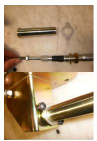
On our new design shifter box: Remove one of the 1" cable nuts from the cable and insert the cable into the hole of the shifter box. Re-install the
