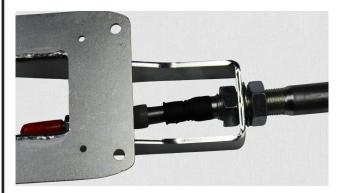
After attachment to cable shifter housing, cycle though all shift points and adjust if shift lever hits the inside of the shifter housing.
