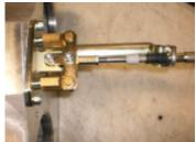
Install boot retaining ring into supplied shifter boot. Attach shifter housing to vehicle floor using supplied 1/4" fasteners. Attach shifter boot to shifter housing using (4) supplied self tapping screws. Install shift knob jam nut and shift knob.
