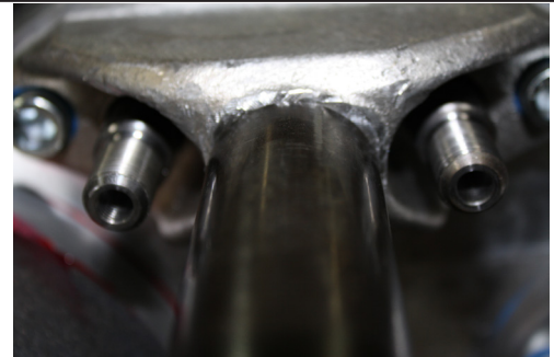
New shift rails with clearance holes drilled
