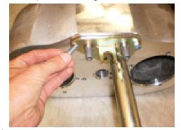
The new brass shift rail ends need to be threaded onto the shift rails. The Igus bushings should be install prior to threading them to the shift rails. Install the brass completely onto the shift rail and then back it off two complete turns, the Igus bushing to be located towards the top of the transfer case.
