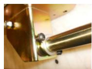
After attachment to cable shifter housing, cycle though all shift points and adjust if shift lever hits the inside of the shifter housing. Install boot retaining ring into supplied shifter boot. Attach shifter housing to vehicle floor using supplied  $\frac{1}{4}$ " fasteners. Attach shifter boot to shifter housing using (4) supplied self tapping screws. Install shift knob jam nut and shift knob.
