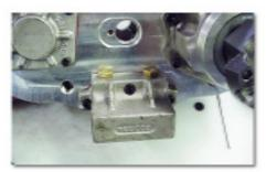
Remove the two thrust washers from inside the case. You should now have access to the shift fork set screws which need to be removed. Remove the three bolts from the shifter control.
