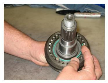
You'll need to install the caged needle bearing back onto the new output shaft along with the high range gear. A new spacer has been included in the kit which fits between the high range gear and the new tapered roller bearing. You can now install the new front retainer over the shaft assembly. Install the new seal washer and the new front yoke with the nut. Torque the nut to 150 ft./lbs. We have also included a new o-ring for the aluminum housing, and this should also be installed now.
