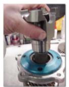
Once the shaft assembly is fully installed, line the 5 retainer bolt holes up with the case and install the 5 fasteners. Make sure you put a dab of RTV blue silicone on the threads and tighten. When you draw up the five front retainer bolts, the race in the rear of the case will be pushed out slightly.
