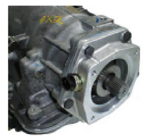
Before tightening the clamp or set screws, trial fit the 51-0405 adapter plate onto the back of the 4L60E transmission. With
