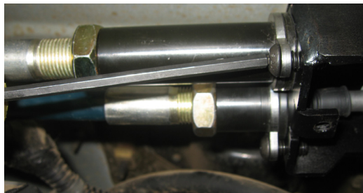
Figure 22: Tighten Retaining Clip
