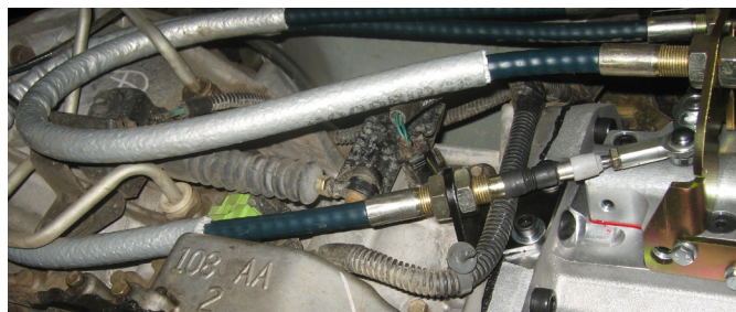
Figure 27: Cable Shifter Routing
