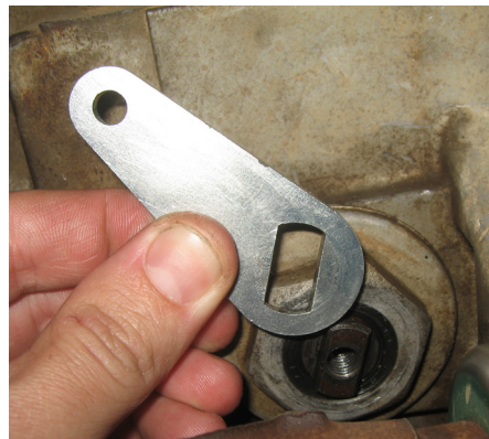
Figure 30: New Transfer Case Shift Lever Orientation NP241
