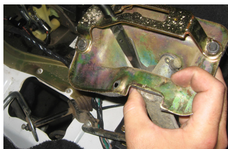
Figure 13: Remove Shifter Linkage
