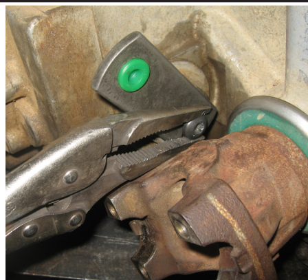
Figure 29: Shift Lever Removal with Needle Nose Vise Grips
