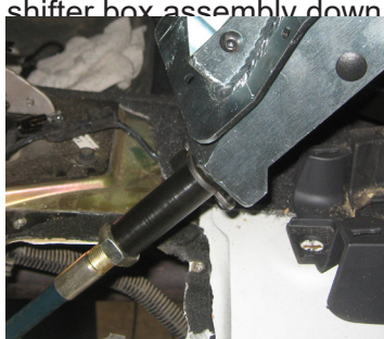
Figure 16: Shifter Box Assembly w/ T-Case Cable
