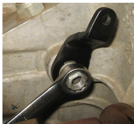
Figure 32: New Transfer Case Shift Lever Orientation NP231
