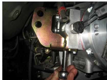
Figure 26: Transfer Case Shifter Bracket
