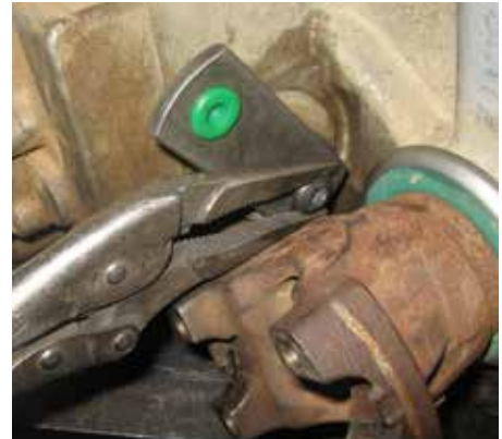
Figure 29: Shift Lever Removal with Needle Nose Vise Grips
