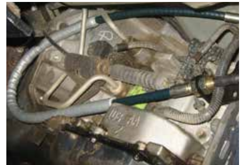
Figure 14: RubiCrawler Cable Routing
