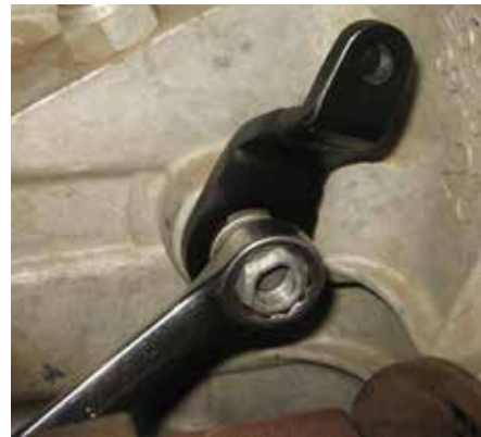
Figure 32: New Transfer Case Shift Lever Orientation NP231
