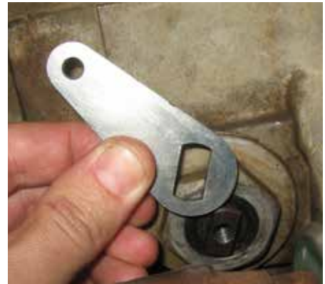
Figure 30: New Transfer Case Shift Lever Orientation NP241
