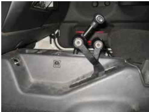
Figure 35: Proper Adjustment with transfer case in 4Low and the RubiCrawler in High
