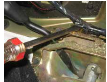
Figure 11: Remove Wire Loom Connector Clip
