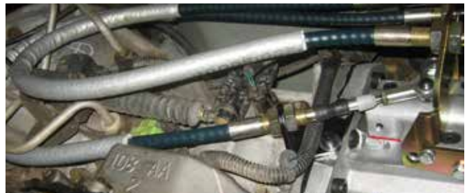
Figure 27: Cable Shifter Routing
