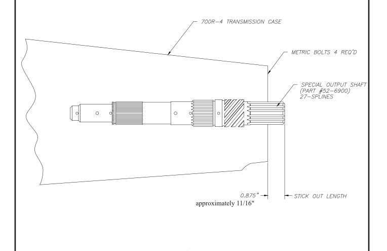
The one piece GM 700R4 output shaft used in this kit is made out of 4340 alloy steel. This output shaft is manufactured with the highest quality materials and standards as the OEM output shaft. The shaft is 11.15" over all in length with 1.68" of spline.
