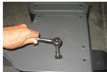
Figure 7: Rear Bolt Location
