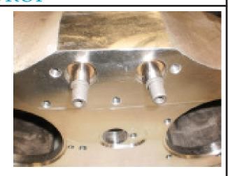
torqued to 35 ft.-lbs. *NOTE:* We manufacture two of these cable mounts, one for a left drop case and one for a right drop case. The mount will only fit the case drop it was designed for.
