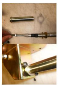
On our new design shifter box: Remove one of the 1" cable nuts from the cable and insert the cable into the hole of the shifter box. Re-install the
