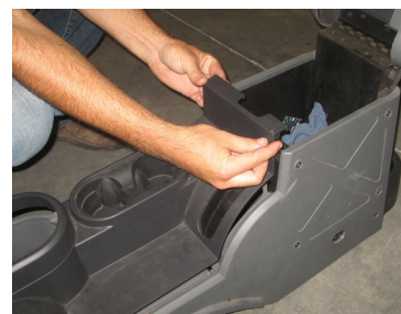
Figure 10: Remove Upper Console
