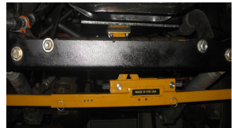
Figure 2: Uni-Raise installation aid
