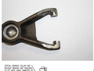
The two photos show the fork gound to fit the new release bearing collar.
