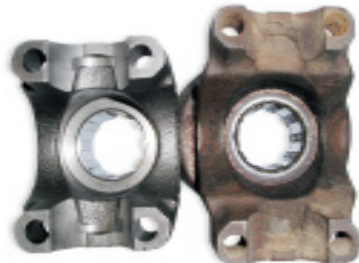
Our new yoke on the left and the stock yoke on the right.
