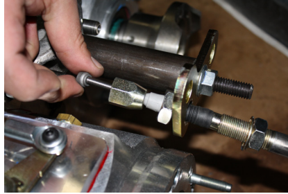
Install the cable nut on the cable threads.
