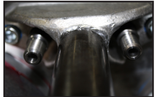
New shift rails with clearance holes drilled
