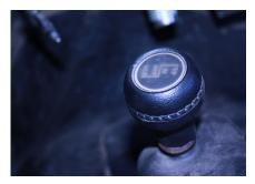
The installation of the 715545 bracket requires you to remove the stock shifter handle. From the applications we have done, this usually means that the bushing between the handle and the shifter gets destroyed. That along with the now worn shift knob (shown above) led us to offer a new handle assembly.
