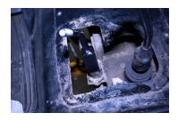
The stock shifter will need the four edges chamfered since the new handle with the tube fitting over this section has radius corners. Grind the edges and then test fit until the handle slides all the way on. The handle is a exact fit with no bushings, just a set screw to lock in place. The handle comes with a new shifter knob that is laser etched with the NP231 shift pattern.
