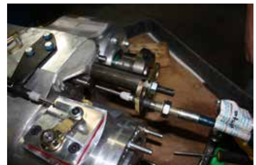
Cable being installed through the bracket
