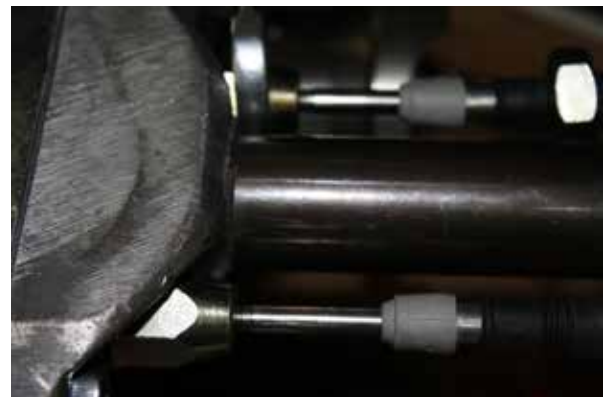
The outer cable housing now needs to be set. Pull the outer housing away from the transfer case. The inner cable should be fully extended.
