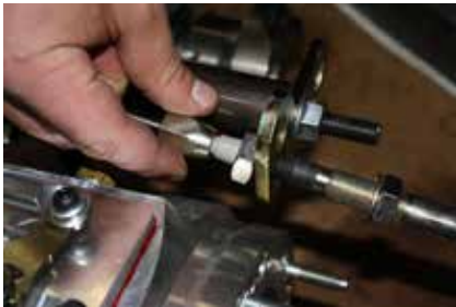
Remove the 1/4" jam nut and install the nut cap over the cable.
