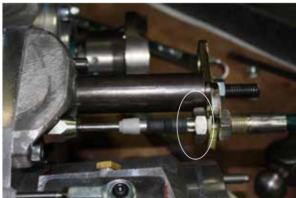
With the cable fully extended in this direction you will now need to secure the 5/8" jam nuts to the bracket of the transfer case. Since the cable has a bit more travel than the Atlas needs, we recommend to thread on the circle nut(photo above) first to the bracket and then give it one addition full turn which will pull the outer cable housing back slightly. Then snug the front nut. Once both nuts are snug to the bracket, tighten them with a wrench. Before moving up to the shifter box shift transfer case back to neutral
