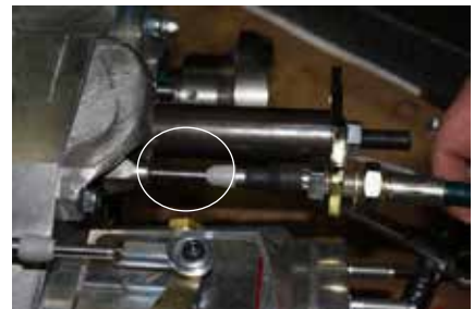
The outer cable housing now needs to be set. Pull the outer housing away from the transfer case. The inner cable should be fully extended.
