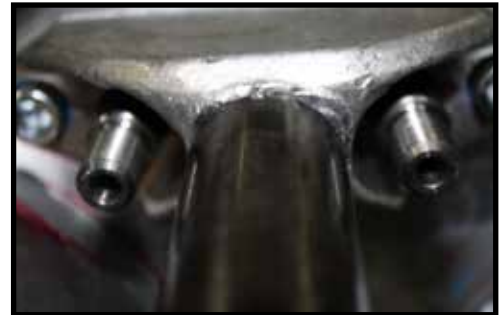
New shift rails with clearance holes drilled
