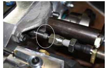
The cable should bottom out in the shift rail and the cable nut should be flush against the face of the shift rail.
