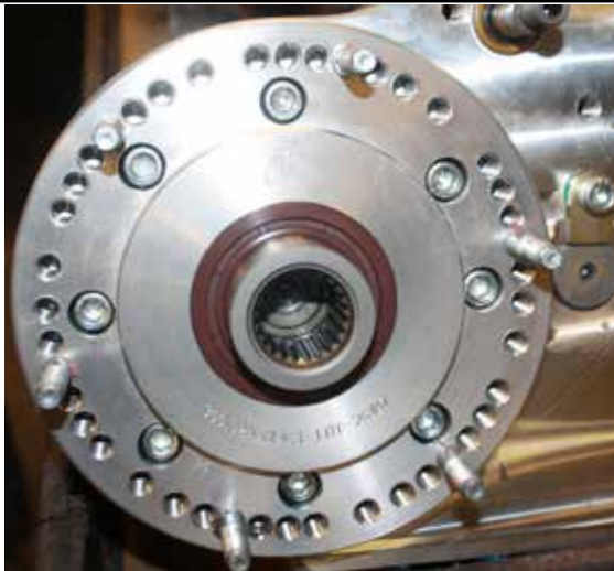
Stud bolts installed for a Jeep JK with the stock rotation.
