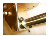
After attachment to cable shifter housing, cycle though all shift points and adjust if shift lever hits the inside of the shifter housing. Install boot retaining ring into supplied shifter boot. Attach shifter housing to vehicle floor using supplied 1/2" fasteners. Attach shifter boot to shifter housing using (4) supplied self tapping screws. Install shift knob iam nut and shift knob.
