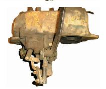
This style shifter requires clearancing when clocking up is desired. Grinding can be done on either shifter housing or SM465 case.
