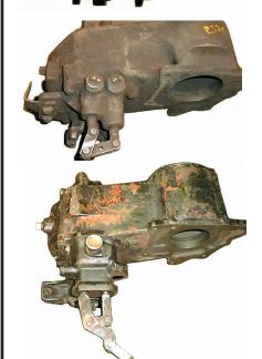
This style shifter can be will allow for installation in any of the three positions. Minor grinding is necessary on the crossmember mount when clocked furthest down.
