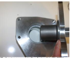
The bearing presses into the adapter plate (51-0801) with a portion protruding though. This portion indexes to the 51-1701 casting to maintain alignment
