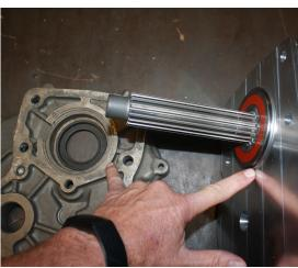
The snap ring and bearing fit into the front of the Toyota transfer case, retaining and indexing the bearing and spud shaft in place.
