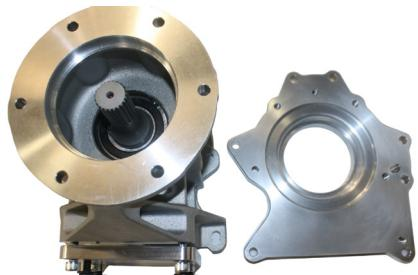
The Jeep 8HP75 have a different support bolt pattern than what were have on our casting plus we add .500" of length with the adapter plate. The aluminum cross member adapter needs to be installed to the housing to align with the modified stock rubber support. See page 3 for modifications needed to the stock support.
