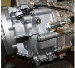
The hole is the correct size for the 16MM x 1.5 tap which matches the thread on the pivot shaft. The plug tap should be around \$20.00. The hole depth on the transmission is approximately .500" which is about the same as the threads on the pivot shaft, we have added a flat washer to be installed under the pivot since the lead of the tap is tapered, not putting full threads in the bottom of the hole.
