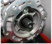
The AX15 has used two different bolt patterns on the tail housing. The photo (left) shown the current pattern. a second pattern of 10 degrees counter clockwise was also used. The adapter to get the TLC transfer case with the proper degree of rotaion requires the other pattern to be added. We offer a clocking ring that will help in drilling the new holes for the AX15, P/N 716516 (shown right)
