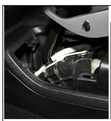
The transfer case lever also has a snap in cover that must be removed.
