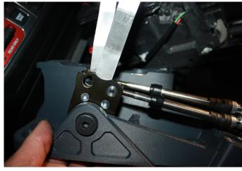
Once cable are secured the base can be installed into the console (Jeep tub) with the new socket head cap screws and washers.
