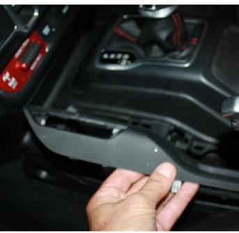
The three plugs that were under the passengers seat need to be pushed under the seat mounting rail and they will allow the console to be lifted. Once the console is removed, the transmission shifter has a small white button that can be pulled out to allow the shifter to be shifter into any gear without the ignition on. Note: the button is spring loaded and will pop back as the lever is shifted.
