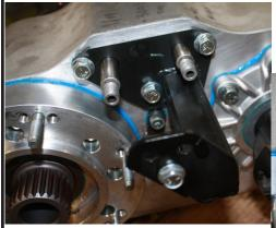
The cable bracket needs to be installed on the front of the Atlas and silicone on the threads of the bolts. Install the retaining nuts until they are fully threaded on the shifter rails.
