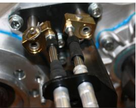
The Atlas is now ready to be installed. We recommend that the Atlas is shifter into gear. This will help line up the input splines of the Atlas with the output splines of the adapter during installation. The photos above show the rear output shifter into high range. Install the Atlas into the Jeep. You can re-install the crossmembers and connect the driveshafts.
