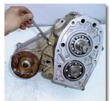
(20) Remove the low range gear by removing the snap ring that retains the roller bearing onto the rear shaft. Press the roller bearing off of the shaft.
