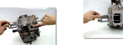
(12) Use a 12mm socket to remove the four bolts that retain the shift fork cover. With a 6mm Allen wrench, remove the shift detent screw plugs found on both sides of the case.
