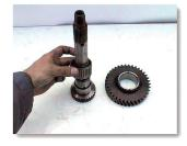
(21) Now that the roller bearing is removed, you will see a spacer. Remove the spacer, the gear and needle bearing.
