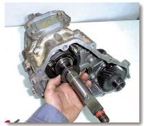
(11) Remove the thick spacer found behind the front wheel drive gear and be aware of the small ball bearing underneath it.
