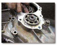
(5) Remove outer bearing C-clip by reaching inside case and pushing up on gear, while lightly tapping on the case with a plastic soft blow mallet.
