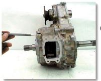
(16) Remove the 4WD indicator switch with a 22mm or adjustable wrench.
