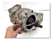
(3) With the rear extension housing removed, you will see the oil pump and speedometer drive gears. Slide the gears off of the rear output shaft.
