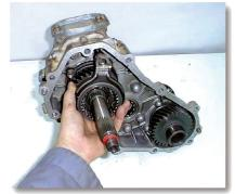
(9) Slide the fork and clutch sleeve off the shift rail.
