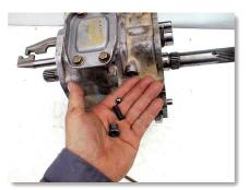
(13) With the screw plugs removed, the shift ball and spring assemblies can be removed from both sides.
