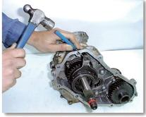
(8) Using a 3/16" (4mm) punch, drive the roll pin out that holds the front wheel drive shift fork.
