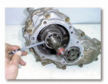
(4) Remove the rear output shaft bearing.
