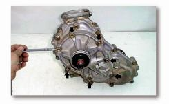
(2) Remove the 7 bolts that retain the rear extension housing with a 14mm metric socket.
