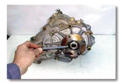
(1) The transfer case must be in 2WD High before starting the disassembly procedures. Remove the nut with a 30mm socket and then remove the flange.
