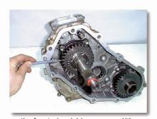
(10) Remove the front wheel drive gear and it's caged needle roller bearing assembly.
