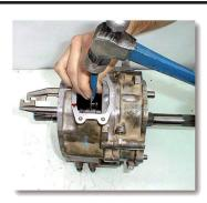
(15) Remove the shift rails, being careful not to lose the interlock pin that might
