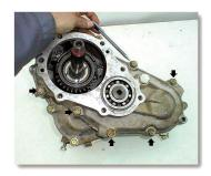
(6) Remove the 10 bolts retaining the rear case cover with a 14mm socket.
