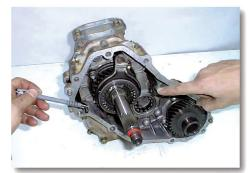
(7) Pull case off. Remove the two lubrication tubes located on either side of the main shaft. **Note their orientation!**
