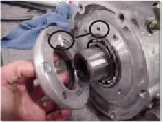
Once you have verified that you have the same style input gear, install the gear into the planetary, install the snap ring. Re-install the planetary assembly into the case and secure the input to the bearing with the front snap ring. **Note:** The only part you should have left out of the case is the old input gear. During reassembly, make sure the oil return hole matches the front retainer hole.
