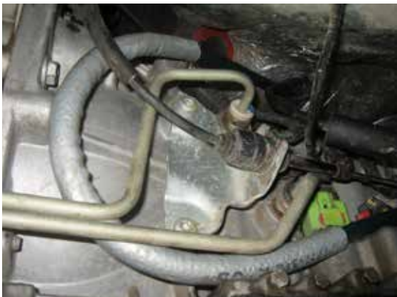
New cable routed along the transmission JK's 2007-11.
