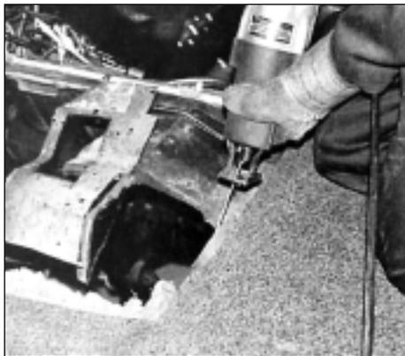
**3** A hole was cut in the floorboard to make room for the overdrive shift lever and allow for the rearward (7-1/2 inch) displacement of the transmission/transfer case assembly and its two shift levers.
