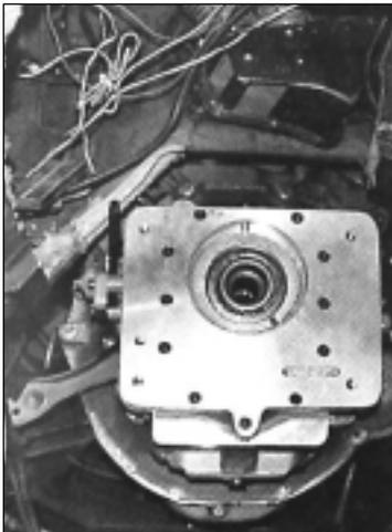
**7** After the Torque Splitter was secured to a transmission jack, it was bolted into place on the bellhousing.
