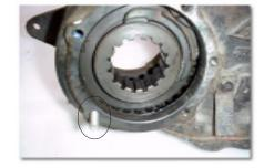
We designed our kit to bolt to the Dana 20 without a gasket. We recommend using a very thin film of RTV blue silicone. Apply a small dab and smooth it out with your finger. Our tailhousing also requires the use of a stud bolt located at approximately 8 o'clock on the case. The stud bolt must be installed so that only .600" is protruding from the case. Make sure the bolt does not go too far into the case and interfere with the Dana 20
