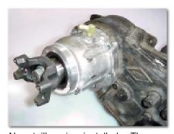
New tailhousing installed. The new bolts need to be torqued to 30ft./lbs. Turn the yoke to make sure the unit is not bound up or is not binding.
