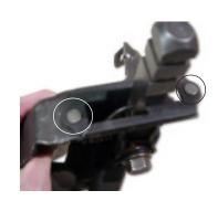
This bracket requires the use of your stock transfer case shifter, the linkage rod to your transfer case, and the shifter gate. All 1987-95 Jeep linkages used a gated shifter that pivoted off of a support bolt. **NOTE:** Some of the Jeep Cherokees used a bellcrank linkage system in which the 715545 bracket should not be used. The stock bellcrank linkage will need to be modified to fit on these vehicles or can possibly use our P/N 715542.
