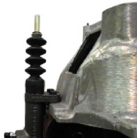
The rear gusset was removed to allow this slave cylinder to mount to the bellhousing.
