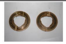
In the racing applications these are the most common areas we see problems with the Atlas. One additional suggestion on regular maintenance is to look at removing the synchro rings, dogs, and springs. Please be aware that the shift block springs must be updated if the synchros are removed, P/N 300395 (2 each) P/N 300396 (2 each).
