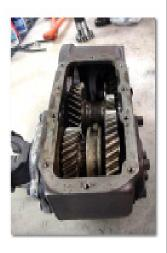
Unbolt and remove the tailhousing. With this removed, you should have the output shaft exposed with the tapered bearing still on the output shaft. This bearing is a tough one to remove. The best way to remove it is by using a bearing puller. Once the bearing is removed, the stock output shaft can be taken out through the front of the transfer case.
