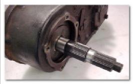
2. Install the shaft through the front of the transfer case, through the slider hub, and onto the stock gear. You should make sure you lube the surface between the gear and shaft. Install the modified thrust washer onto the output shaft. This thrust washer is required to obtain proper gear and slider alignment with the other components in the transfer case.
