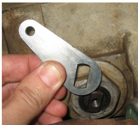
Figure 30: New Transfer Case Shift Lever Orientation
