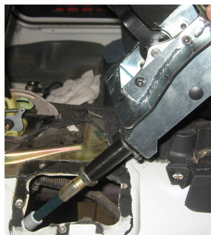
Shifter Box Assembly w/ T-Case Cable
