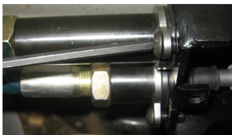
Figure 22: Tighten Retaining Clip
