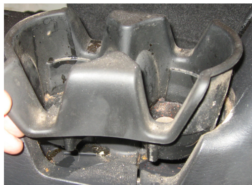
Figure 8: Cup Holder Removal
