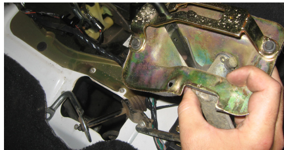
Figure 13: Remove Shifter Linkage
