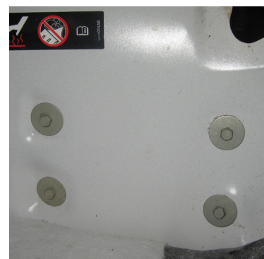
Figure 12: Shifter Pivot Assembly Bolts
