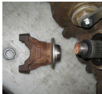
Figure 31: Proper Yoke Installation Order
