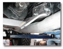
Due to tight tolerances, the crossmember holes to the frame have been oversized to allow for some adjustment. We have also slotted the holes in the crossmember tube to allow for some vehicle variances.
