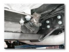
NOTE: The center of the rear output yoke should be 12.46" from the drivers side inner frame rail.
