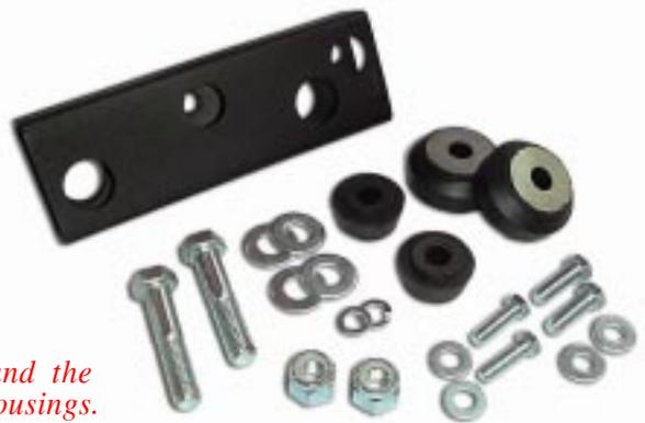
**NOTE:** *This transmission support mount is designed around the use of the Advance Adapter transmission to transfer case housings.*
