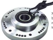
Newer Atlas T/C's use a bolt on bearing reaing retainer, this snap ring is not used. the bolts are torqued to 150 In.lbs.
