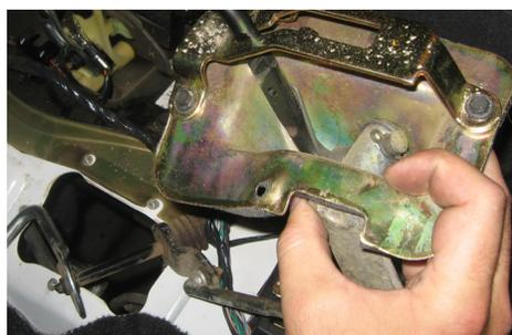
*Figure 13: Remove Shifter Linkage*
