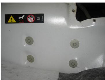
*Figure 12: Shifter Pivot Assembly Bolts*
