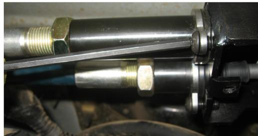
*Figure 22: Tighten Retaining Clip*
