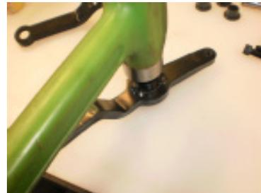
The Igus bushings must be **pressed** into the shift handles. A arbor press or a light hand with a hammer works well. Once the bushings are installed the pivot pin gets installed through the handles with the wave washer between them.
