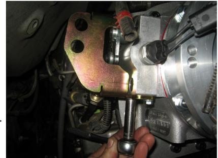
*Figure 26: Transfer Case Shifter Bracket*
