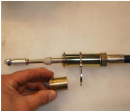
Install the short cable barrel and then mount to the shifter housing. Align the heim joint with the access hole on the shifter housing and the handle, then bolt together with the button head bolt. The plastic cap can be installed after.
