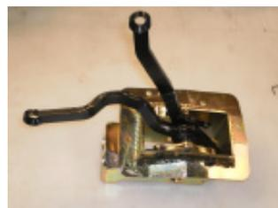
Slide the pivot pin mounts over the pivot pin, make sure the pivot pin is flush with the outside of the pivot pin mount. Use the small set screw to lock the pin to the mount. Check the orientation of the handles and set the handle assembly into the shifter housing, the one socket head bolt mounts the rear pivot pin mount to the housing and the other three holes use button head bolts.
