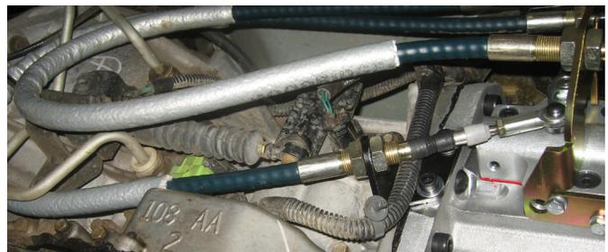
*Figure 27: Cable Shifter Routing*
