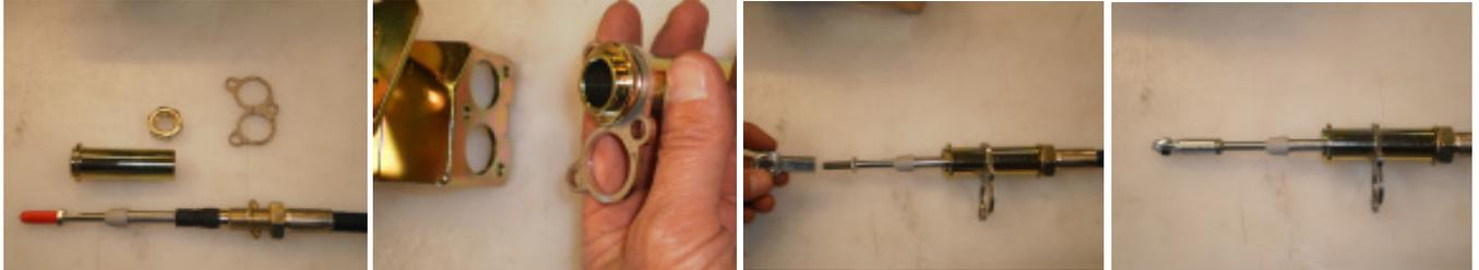
Remove the double nuts on one end of the cable and install the heat shield. Reinstall one of the nuts and the star washer. Take the long barrel retainer and slide the retainer on it, verify the retainer is orientated correctly to bolt to the shifter body. Thread the barrel onto the cable and then install the heim joint to the cable end.
