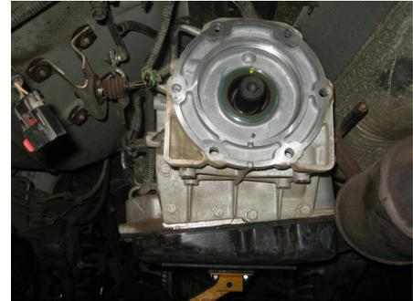
*Figure 5: Transmission Tailhousing*
