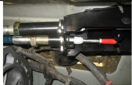
*Figure 18: Barrel Mount*
