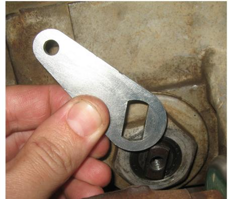
*Figure 30: New Transfer Case Shift Lever Orientation NP241*
