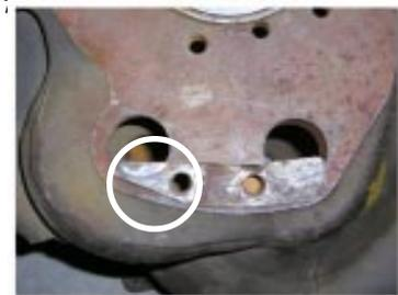
Some transmissions may require a modification to the cluster pin / reverse idler pin retaining bar. There are several different styles of this bar and a few will interfere with the mounting of our adapter plate to the transmission. Before final assembly, check the adapter plate for clearance and modify the retaining bar if necessary.
