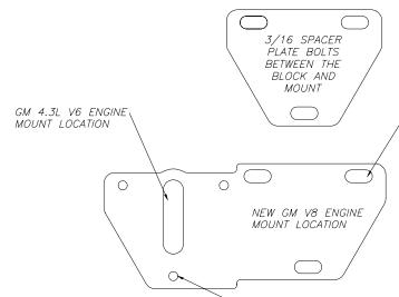
,BOLT ENGINE PLATE TO GM V8 USING.390" 3/8-16 x 1 1/4" LG H.H.S. (PART #723722) GRADE #5 w/ F/W & L/W. SLOTTED HOLES TO PROVIDE LATERAL ADJUSTMENT.
