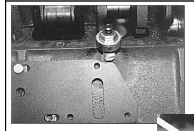
**NOTE:** If you are using a late model block that utilizes an engine block sensor, you will need to purchase a Brass Street Elbow, Dorman Part #490-117. This will allow you to retain your sensor in the original location in order for the block to operate correctly.
