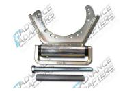
We have provided a crossmember plate if you choose to use a stock transmission rubber support. This plate bolts to our adapter using the two 3/4" long bolts. The stock rubber support would then be installed on top of this plate with the two support bolts going through the rubber support and our support plate holes, and threaded into the transmission.
